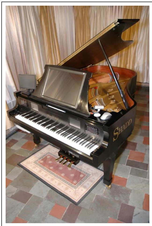
Figure 1. Prototype piano modified for neurodevelopmental disabilities—7'2" Semi-Concert Grand. Enhancements visible in the figure include 4 liquid crystal display (LCD) touch screens (with 3 embedded and 1 stand-alone monitor) for interaction with the onboard computer and software, a mouse (and alphanumeric keyboard stowed beneath the keys), a fourth pedal for page turning, video camera to facilitate remote communication, embedded speakers above the keys facing the player, and electronic data ports beneath the upper keys that allow the piano to interface with additional tools and systems.
